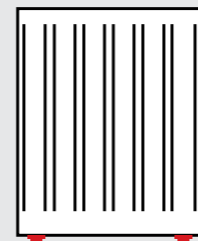
REF. 004 Welded feet for extra stability (maximum 1100mm high radiator)
